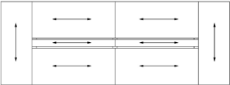
Grain Direction for Double Sided Benches and End of Run Worksurfaces
